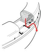
Patented Air Flow Control technology delivers optimal passive attenuation across all frequencies, without increasing earcup size or weight. A patented baseplate chamber and high-tech non-woven layer manage the flow of air inside the earmuff to control how sound reaches the ear. The result is better, more consistent overall attenuation for virtually all industrial noise environments.
