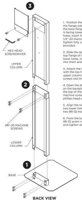
1. Position the base in the desired location with the flange side up. Slide the lower column over the base flange so the open face of the column is facing towards the back. Align the four lower holes, insert four
